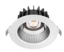
ELIA AL is a flush-mounting LED device for accent lighting in commercial areas and offices, composed of a white powder-coated die-cast aluminium frame and 2 different optics (36° and 60°) that guarantee a UGR of less than 19. The range is available in two sizes, with a colour temperature of 3,000K (warm white) or 4,000K (neutral white), a colour rendering index of more than 80 or more than 90 and the option of an electronic power supply with On/Off or DALI command.
